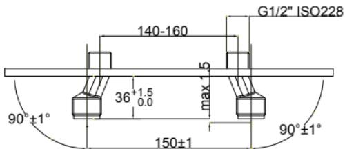
Adapt the inter-axial distance to that of the armature and adjust them both to the same height.
