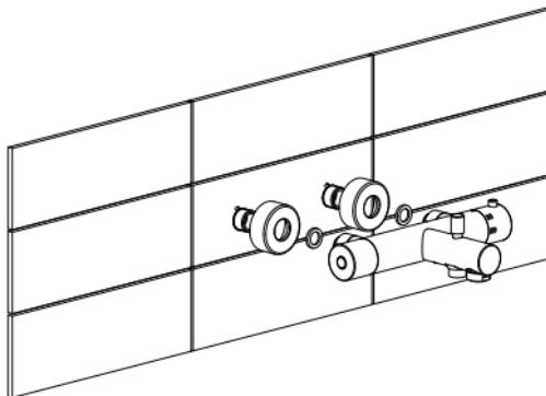
Insert the gaskets into the nuts and attach the armature by means of a 30 mm fork key, check the tightness of the gaskets.
